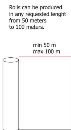
Rolls can be produced in any requested lenght from 50 meters to 100 meters.
