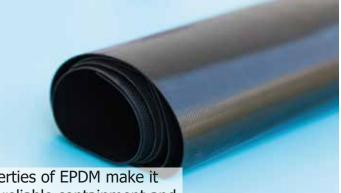
The versatility, durability, and waterproofing properties of EPDM make it suitable for a wide range of applications requiring reliable containment and protection against water and contaminants.
